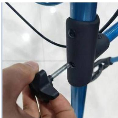
Repeat this operation at the back by inserting the rear legs into the back frame on both sides, then secure with the knobs.
