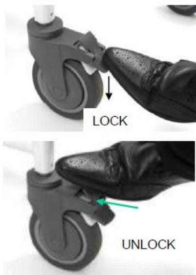
The castors can be locked so that the castor wheel cannot move forwards or reverse, nor will the castor wheel swivel. To lock the brakes, press down on the locking tab as shown on the left. To unlock the brake, press on the section of the tab that has been raised.
