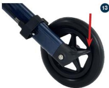
We recommend you use our built-in, kerb climber (see figure 13). This saves you lifting the rollator over obstacles such as thresholds and kerbs. Just step down on the kerb climber and with a gentle pull back on the handles, the rollator will raise its front wheels to easily maneuver over obstacles.
