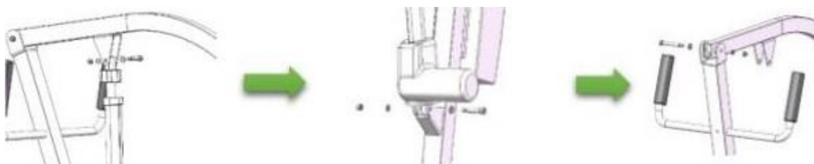
Fig. 3. Installation of lift arm
