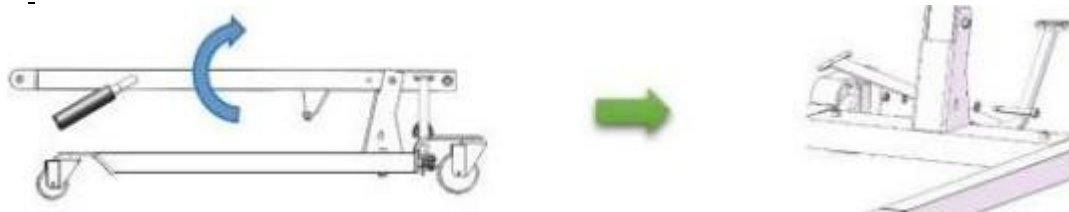
Fig. 2. Scheme of mounting the lifting column.
