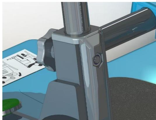
7. When both sides of the lower leg frame are securely fastened to the base, position the lower leg support assembly over the top of the tubes
