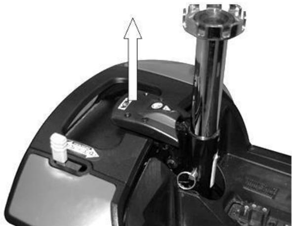
To reassemble, allow the rear section of the scooter to rest upside down on the anti-tip wheels. Lift the front section by the seat post towards the rear and place the 'ears' on either side of the frame over the main tube of the rear section as shown below. The front section can now be gently lowered into position.
