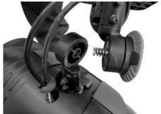
There are two electrical connections - white and black plugs. These must be connected to the corresponding coloured connector. Once connected, carefully push the connectors one by one through the hole in the chassis cover and insert the eyelet.
