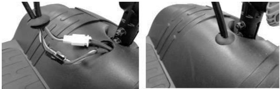
To fit the seat post, the rear of the scooter must be removed to gain access to the fixing bolt. Locate the seat post and align the holes in the frame and upright at the desired height. Tighten the bolt using the Allen key and the spanner supplied. Refit the rear of the scooter.
