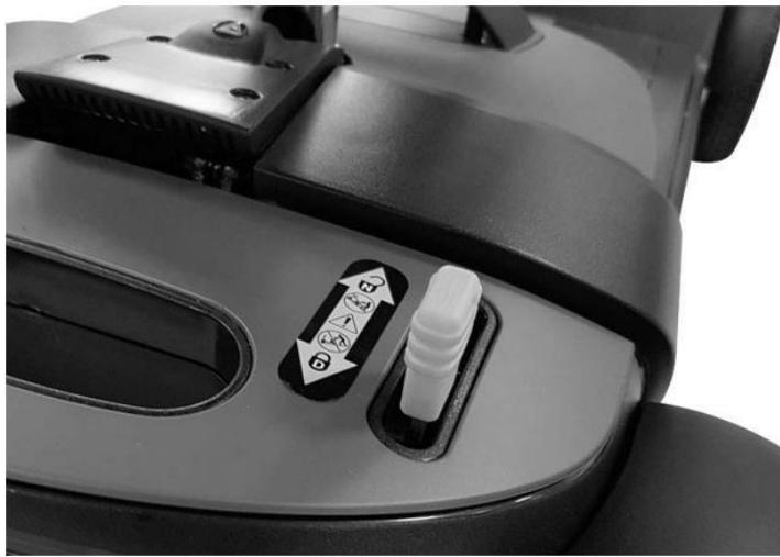
**Caution!** Never leave the scooter unattended in freewheel mode, as it may roll down a slope. Freewheel mode should only be used in an emergency to move the scooter due to a breakdown. NEVER move the scooter in this mode when it is occupied. NEVER tow the scooter.
