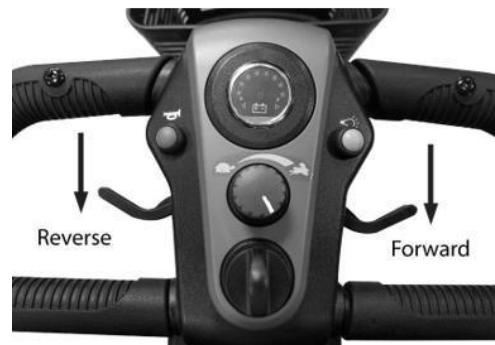
The speed and direction of the scooter are controlled by the accelerator lever. The arrows in the image above indicate the direction in which the scooter will move when the lever is operated as shown.
