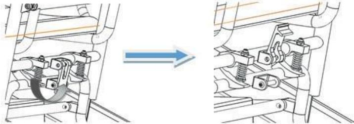
Step 2: Compress the backrest tube to completely folded
