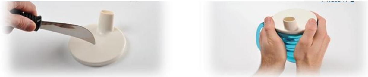
PP (Polypropylene) is an injection-molded thermoplastic. This material offers excellent heat resistance and very good impact resistance. Compared to PETG, it is more prone to scratches and staining from certain foods and drinks, but still delivers solid performance.
